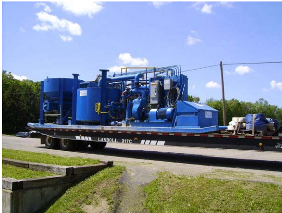
Fig. 12 Slurry Batch Plant
