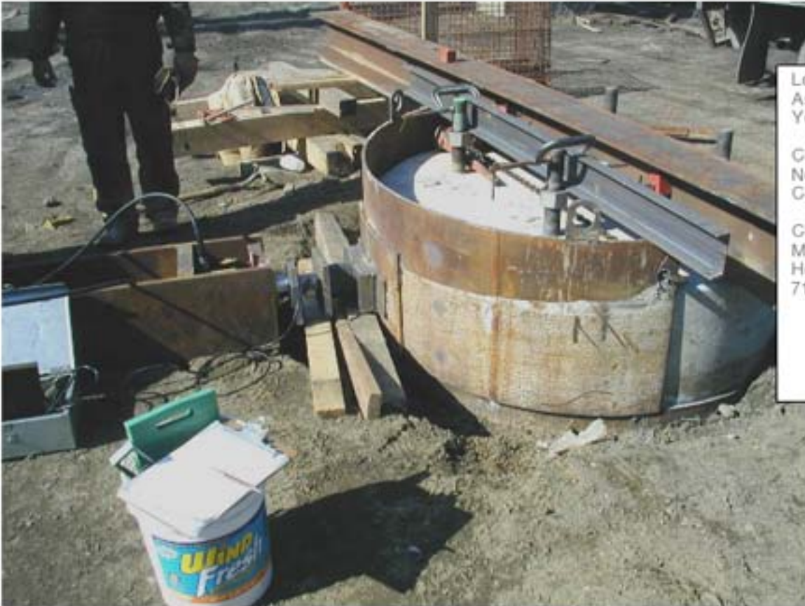
Jack and Deformation Measuring Setup for Lateral Load Test on Drilled Shaft
