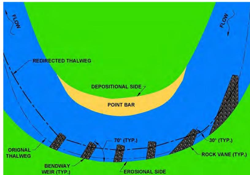
**Figure 1 – Typical stream reach with river training structures**
